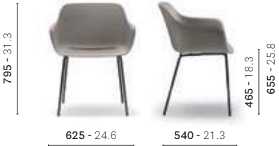
2734R Armchair, recycled polypropylene shell, steel tube frame
