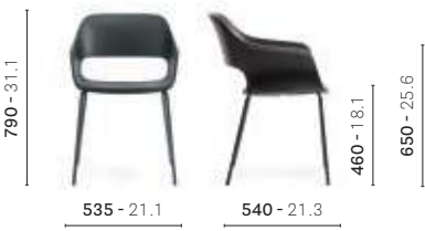
2735 Armchair, polypropylene shell, steel tube frame
